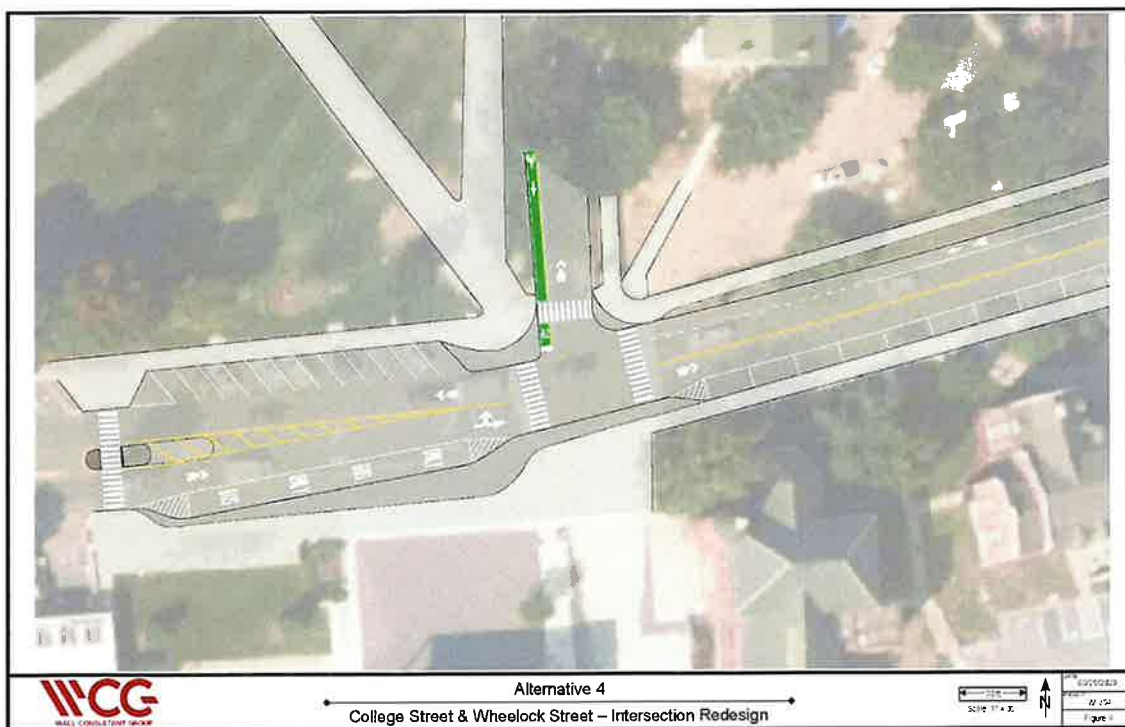
FIGURE 2: PREFERRED ALTERNATIVE (ALTERNATIVE 4 - REDESIGNED SMALLER INTERSECTION)
