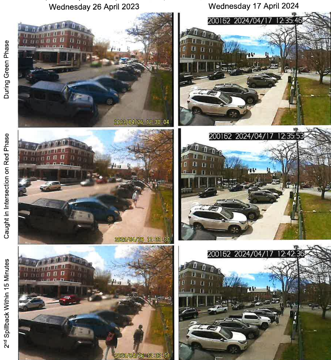
FIGURE 5: QUEUE SPILLBACK TO AND THROUGH THE MAIN STREET & WHEELOCK STREET INTERSECTION, BEFORE (APRIL 2023) AND DURING (APRIL 2024) THE PILOT
