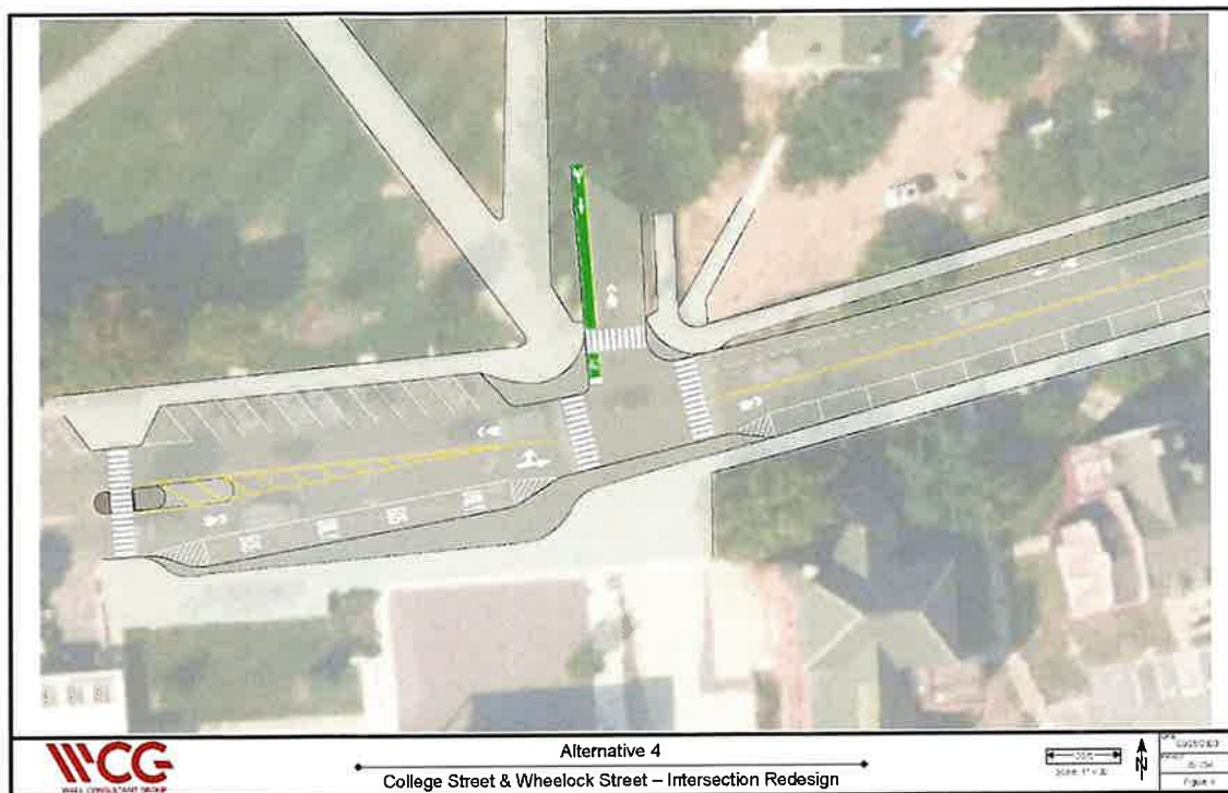
FIGURE 2: PREFERRED ALTERNATIVE (ALTERNATIVE 4 - REDESIGNED SMALLER INTERSECTION)
