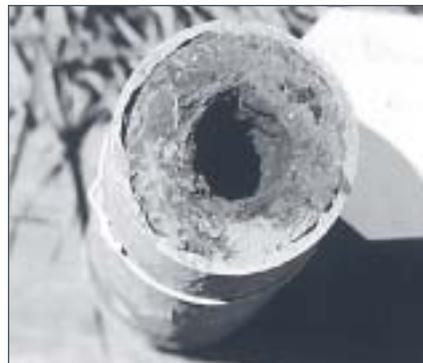
Current State of a Pipe Installed in 1893
